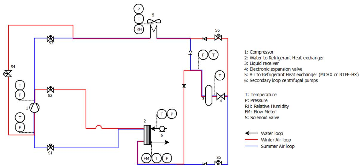
**Figure 1:** Layout of the heat pump prototype during tests. Blue lines represent the refrigerant circuitry for the summer-air mode, red lines for the winter-air mode. Black lines represent the water circuit. Additional heat exchangers are not reported here.
