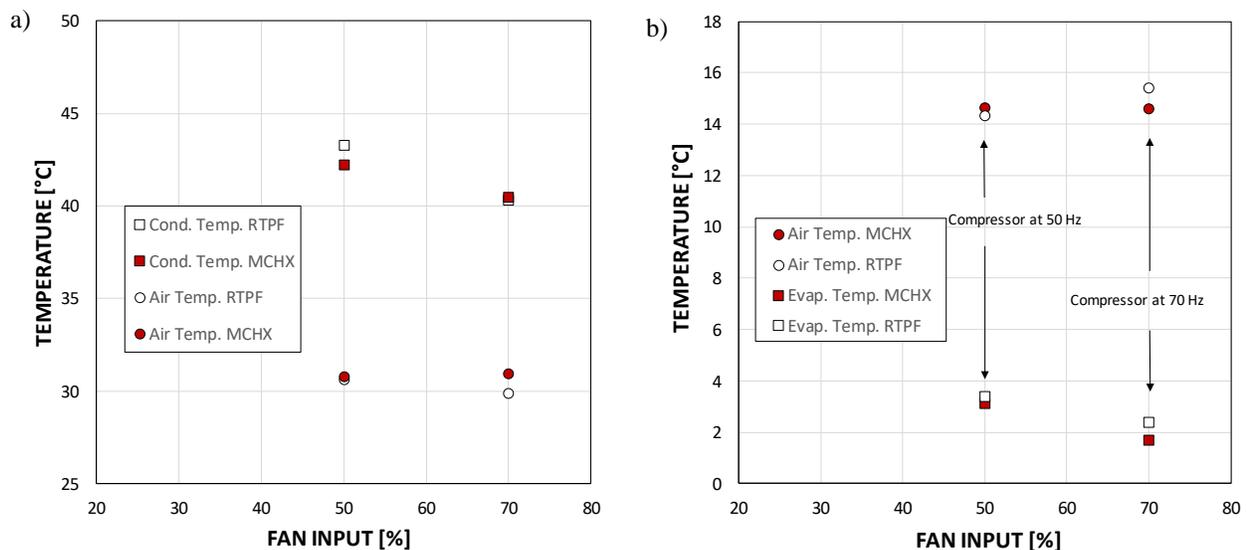
**Figure 3:** Comparison between the RTPF-HX and the MCHX (a) in summer air-mode at variable fan speed and fixed compressor frequency (50 Hz) and (b) in winter air mode at variable fan speed and variable compressor frequency (50 Hz when fan is at 50% and 70 Hz when fan is at 70%)
