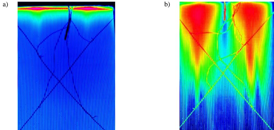
**Figure 4:** IR camera images of the MCHX taken during the experimental tests: a) working as condenser (fan at 50% and compressor at 70 Hz); b) working as evaporator (fan at 50% and compressor at 50 Hz).
